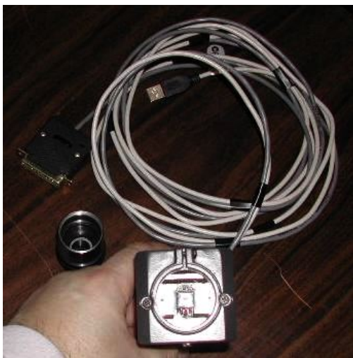
Figure 3: Front View with the Eyepiece focuser adapter removed.
