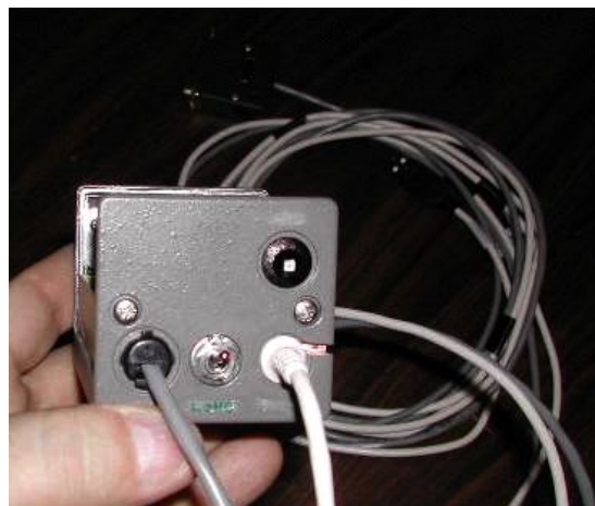
Figure 6: Rear Panel, Parallel (bottom left), Long Exposure switch (bottom middle), USB (bottom right), LED (top right).
