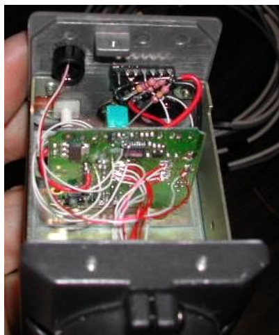
Figure 5: Close up of the wires going to the ToUcam PCB.
