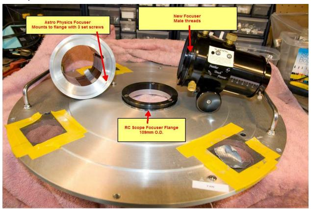
As it turns out, the focuser and retaining collar have a very tight tolerance and a small scratch on the focuser retaining sleeve is all it took to cause it to jam. A quick spin on the lathe took care of that.
