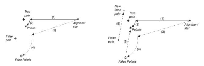
Note also that movement (4) is the correct *angular* revolution, but it is part of a circle around the false pole instead of the true pole. Then the user adjusts the mount, performing movement (5): This movement superimposes the false Polaris on the true Polaris. It also moves the false pole closer to the true pole, *which is the object of the game*.
